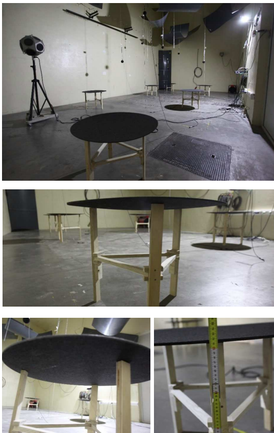
Photos top to bottom from measurement 3: Superloop plus 70 - height 50 cm
